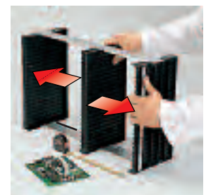
shifting the central divider
